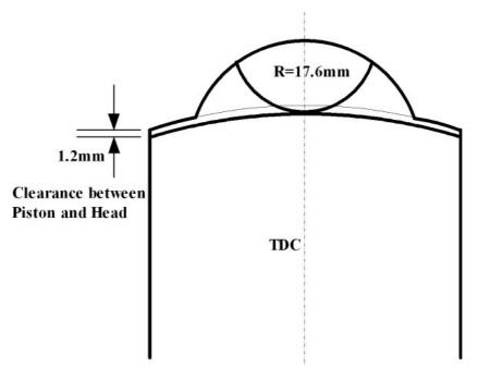
At 10 degrees after TDC the hemisphere of the chamber is almost fully enflamed and the flame front is on the point of moving into the squish area. As can be seen the squish area is rapidly opening up and will be experiencing reverse flow.
