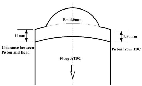
This is still way before the exhaust port opens which points to the fact that for burning mixture to exit the exhaust port something serious has to be wrong with the combustion process.
